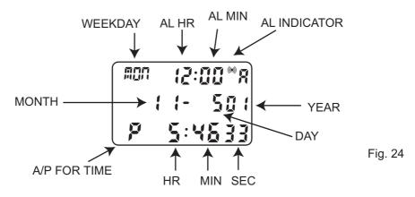
Press and hold B button will go into the TIME SET mode with the AL HOUR blinking. Press A to set the AL HOUR. Press B to select digits in the following sequence: AL HR, AL MIN first digit, AL MIN 2nd digit, AL OFF/ON, YEAR last digit, YEAR 1st digit, MONTH, DATE, 12/24HR selection, HOUR, MIN 1st digit, MIN 2nd digit, and SECONDS. Press A to set the blinking digits.
