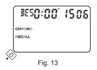
The AVERAGE calculation and BEST record do not take into account the last section of time before STOP. Therefore, in order for the stopwatch to keep track of the average and best records of all Laps, always use the B button until the end of the race. Pressing D again will go to the next race records or return to the 1st race records (if there is no further race).
